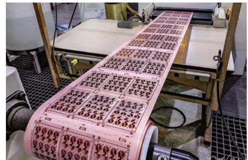
*Novaclad™ HDI offers single and double-layer flexible interconnects that thrive under extreme conditions in electronic applications.*
